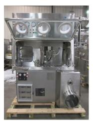
side discharge with pneumatic plug valve with controls, unit mounted in Howorth isolator, single sided with (3) gloves, side bottom discharge section with (1) glove with controls, Aeromatic-Fielder serial# 8453, Howorth serial# 04128-2.
