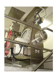
with 20" diameter rear mounted drum unloading system with drum clamp and lift assist, stainless steel IBC included, serial# C70269, built 2007.
