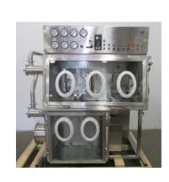
isolator, stainless steel construction, single sided, with (3) gloves main section, bottom discharge section with (2) gloves, back mounted anti chamber with (1) glove, with blowers and controls, Fitzmill serial# 1546, Howorth serial# 04109/1.
