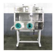
antechamber), with (2) glove ports, antechamber measures 12" wide x 15" high x 12" deep, with 11" x 11" inlet and outlet, with (2) 4" vents on side, on adjustable height cart, 120 volt, serial# 0997-4P.
