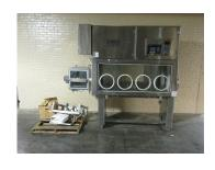
coupled 20 hp, 230/460 volt xp motor with vfd controller mounted in xp panel, unit mounted in Carlisle Life Science isolator, stainless steel construction, single sided with (5) glove ports, approximately 60" long x 22" deep x 43" high, with 10" diameter end access door, on stand.
