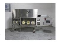
single sided with 3 glove ports, approximately 30" wide x 16" deep x 23" high anti chamber with 2 glove ports, with blower, order# C999511, built 1999.
