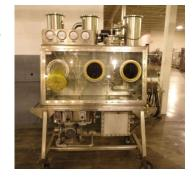
single sided, (3) glove ports with 1 hp, 115/230 volt blower, 15" end access, on stand, XP design, serial# 5008-A, built 1993.
