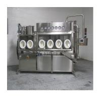
and pass thru opening, 22" wide x 64" long main chamber with (4) gloves, single sided, 15" diameter back access with door, multiple HEPA filter housings, Allen Bradley controls, 480 volt, serial# 30700C0600, Built 2011.
