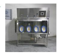
door access, 13" diameter end access, with Allen Bradley Micrologix 1500 plc controls and blower, on stand, serial# 33279-2, built 2005.
