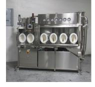
and pass thru opening, 22" wide x 64" long main chamber with (4) gloves, single sided, 15" diameter back access with door, multiple HEPA filter housings, Allen Bradley controls, 480 volt, serial# 30800C0601, Built 2011.
