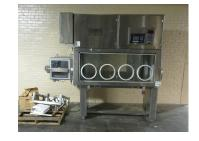
high inside chamber, single sided, 6 gloves with side access door, (2) 16" X 29" side access doors, 18" bottom outlet with cover, 4" bottom outlet with cover, CIP spray balls, (2) top mounted internal lights, 1 hp, 230/460 volt blower, on stainless steel stands with control panel, serial# 4344-200, new 2009.
