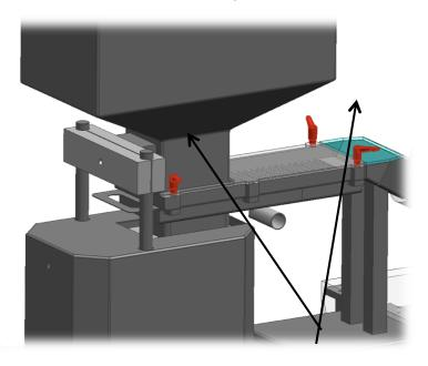
Loosen 2 handles on each side to remove sieve plate
