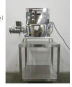
Used LCI Fuji Paudal Marumerizer, model QJ-230T, stainless steel constructin, 230 mm diameter disk, jacketed bowl on base with approximately 1 hp motor, serial# 4100754, built 2007.
